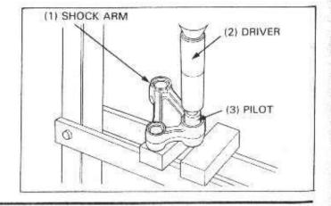
Pack new needle bearings with grease.
