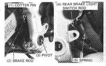
Apply grease to the pivot and install the removed parts in the reverse order of removal.
