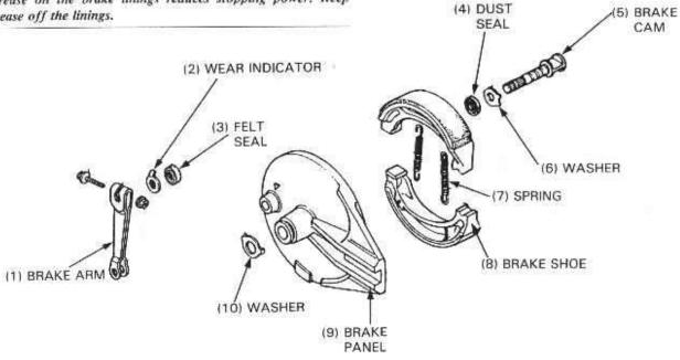
Install the washer onto the brake panel by aligning the groove with the boss of the brake panel.
