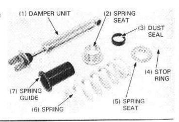
Visually inspect the damper unit for dents, oil leaks or other faults. Replace the damper unit if necessary.
