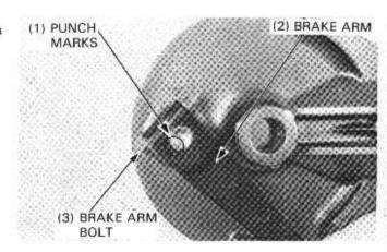
Install the new brake shoes on the brake panel. Place the brake panel assembly in the wheel. Install the rear wheel (page 13-8).
