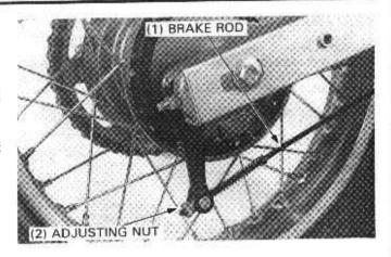
Loosen the rear axle nut.
