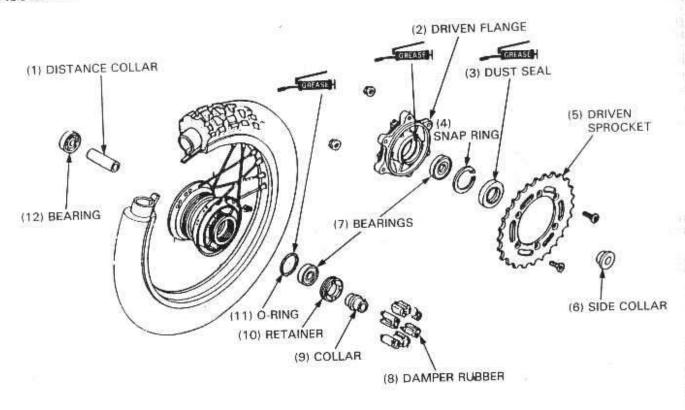
Pack the bearing cavities with grease.
