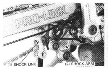
Tighten the shock link-to-swingarm bolt.
