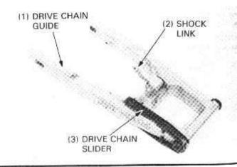
Set the swingarm in the frame and install and tighten the pivot bolt.
