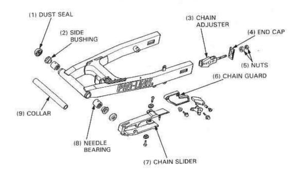
Press each side's bearing and bushing into the swingarm totogether using hydraulic press.
