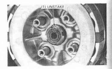
Install the clutch center holder as shown, and remove the clutch lock nut.
