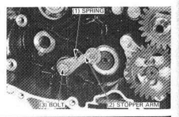
Assemble the stopper arm, bolt, washer and spring then install them in the case.
