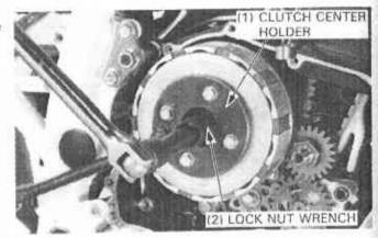
Remove the lock washer, clutch center and discs.
