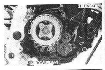
Install and tighten the crankcase cover bolts, except at the clutch cable holder, in 2 or 3 steps in a crisscross cattern.
